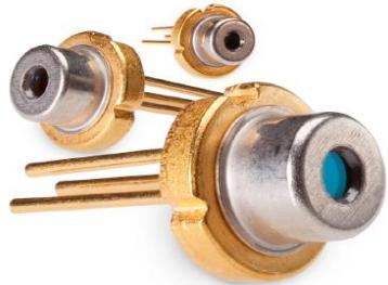
**FVLD-420-120S** is a single mode laser diode with 120mW CW output power at 420nm. It is supplied in a 5.6mm TO can with Photo Diode and Zener Diode. The laser diode is suitable for the use in various opto-electronic applications.
